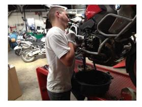
After a brainstorming session, the workshop manager, Cedric, goes to the showroom and returns with a brand spanking new GS, and proceeds to take out the fuel tank. Changing the tanks finally solved the problem, and we realized that even though the fuel pump was running, it obviously was not delivering the right pressure. New fuel pump installed, and all is well!
